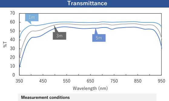
Light guide bundle with 5 mm diameter (Single fiber diameter: 50  $\mu$  m)
