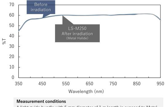
A light guide bundle with 5 mm diameter of 1 m length is exposed to Metal Halide Lamp (400 nm Cut Longpass Filter) for 100 hours.
