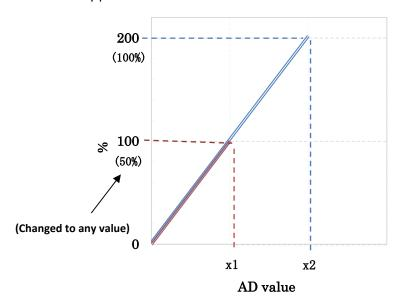
For example, in case the light intensity mode is set at "Por", after a certain amount of incoming light is taught, set the light intensity as 100% value when the AD value is x1, and change the 100% value to 50% with this function, 50% will be displayed when the AD value is at x1 and 100% will be displayed when the AD value is at x2 in the monitor operation.
